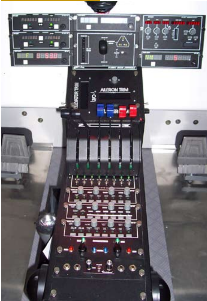
The centre console features an interchangeable throttle quadrant to reflect the aircraft type being flown. (FSAP)
